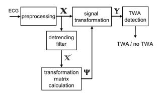
Fig. 2. Block diagram of the multilead scheme.
